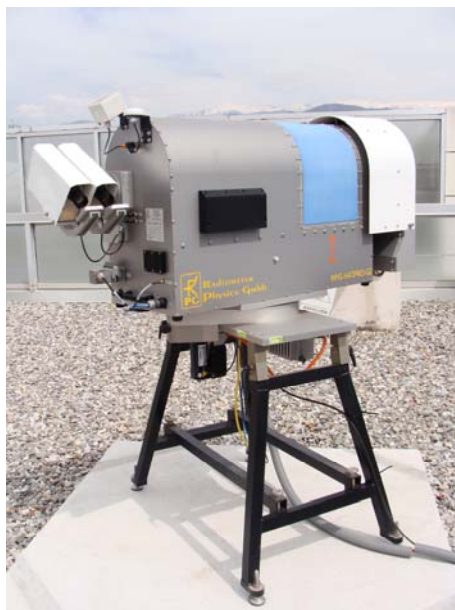
Figure 3.8. Microwave radiometer HATPRO system operated at the Granada station.
