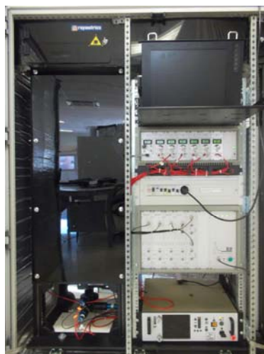
Figure 3.1. Raman lidar system operated at the Granada station.
