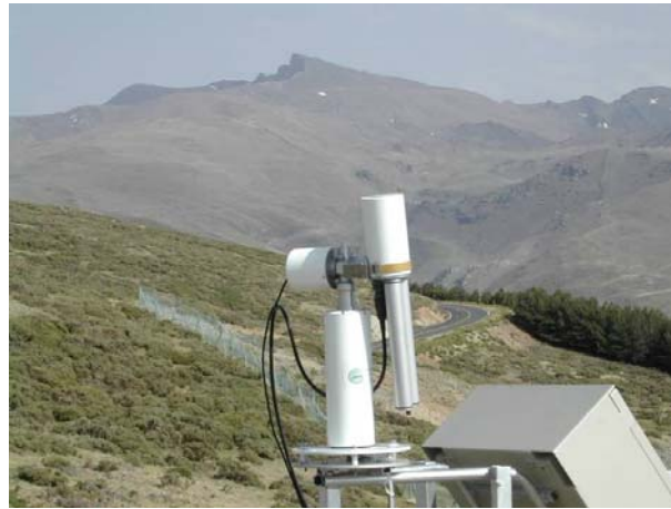
Figure 3.5. A Cimel CE 318-4 fielded at Sierra Nevada (Granada, Spain)
