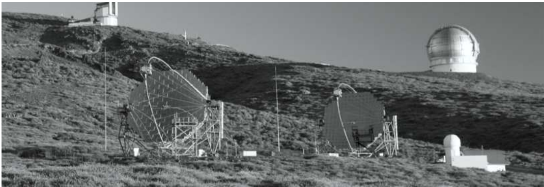
Fig. 1 The MAGIC array of two 17 m diameter Cherenkov telescopes, located in the Canary Island La Palma.
