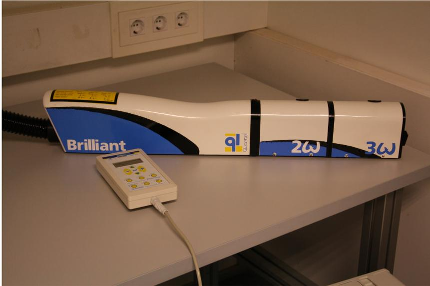
Figure 3.2: Brilliant Nd-YAG 1024nm laser acquired by IFAE with second and third harmonic generators at 532 nm and 355 nm respectively.
