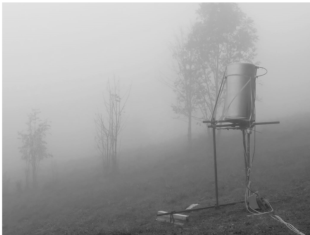
Figure 5.4: The sampling setup at the Otlica Observatory in working conditions. The inverted metal container served as an interstitial inlet, which, in combination with the BioSampler, was used for the collection of particles smaller than 5 \mu\text{m} .
