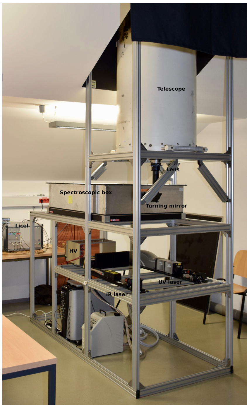
Figure 5.2: Assembled lidar system in its working environment at the Center for atmospheric research of the University of Nova Gorica in Ajdovščina. The atmosphere is accessed through a 1\text{ m}^2 rooftop window with > 85\% light transmission and an electrical shutter. The telescope is mounted as close to the window as possible, leaving room for the spectroscopic filter and the transmitter below. In addition, panels painted in black are covering most of the mount to prevent any additional stray light from the room to get into the lidar, as well as to prevent any laser beam scattering around the room the system is built in.
