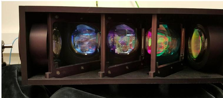
**Figure 10.8:** Polychromator design layout (*top*) and picture of the interior (*bottom*) for a 4-channel read-out unit.
