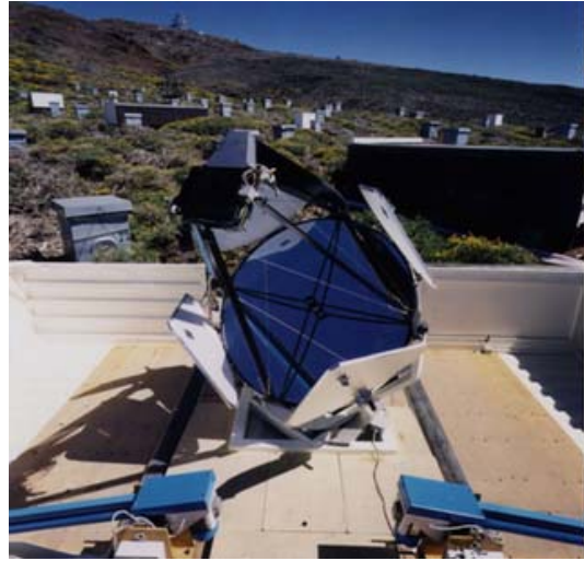
Figure 1: Picture of the CLUE telescope and the foldable container when it was operating in La Palma (Spain). The telescope will be re-designed as Raman LIDAR.
