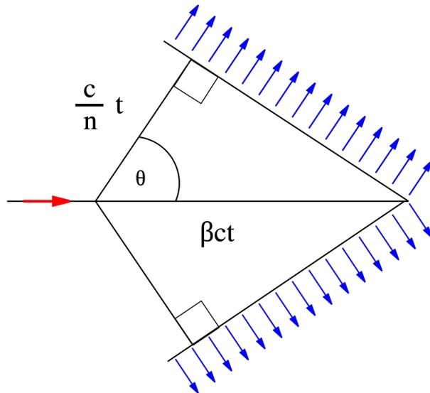
Figure 2: Figure extracted from Wikimedia Commons that shows how Cherenkov radiation is produced along dipole wavefront.
