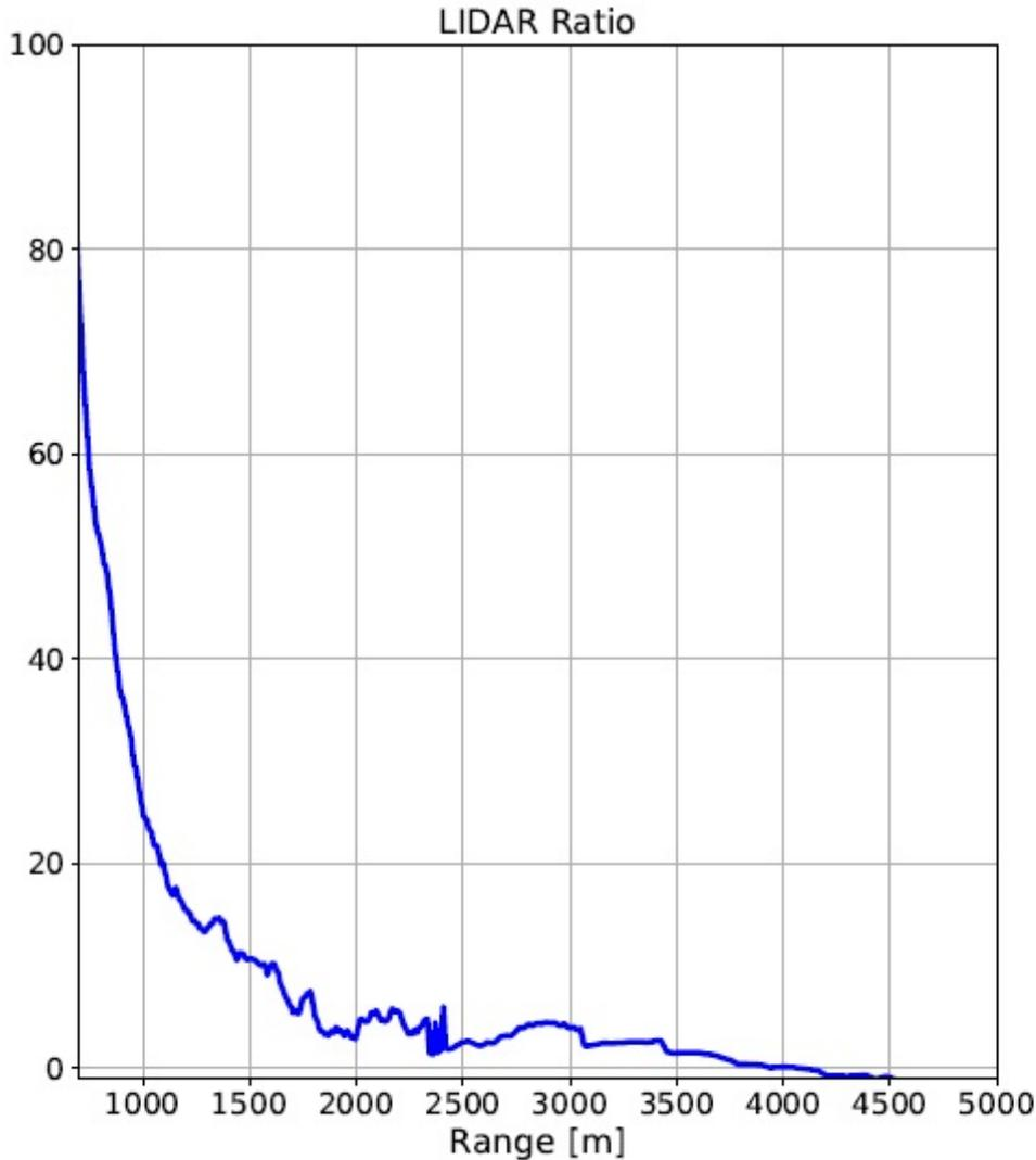
Figure 10: The LIDAR ratio evolution as a function of altitude of atmosphere above the UAB campus obtained through extinction and backscattering coefficients.
