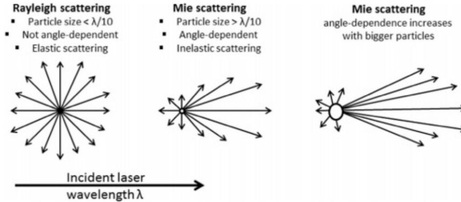
Figure 7: Schematic showing the differences between Rayleigh and Mie Scattering depending on the particle shape. [16]
