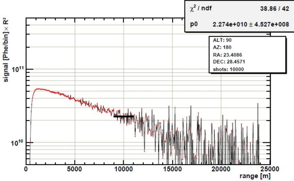
Figure 5: An standard clean night atmospheric signal profile from an elastic backscatter channel. [12]
