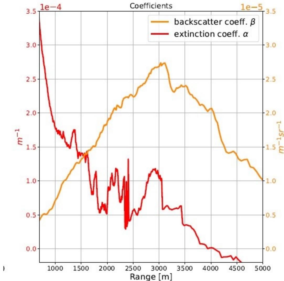
Figure 9: The extinction and backscattering coefficients evolution as a function of altitude of atmosphere at the UAB campus.
