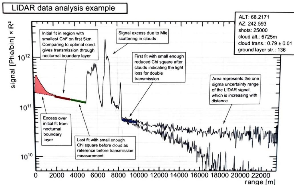
Figure 4: An example of a range-corrected signal from an elastic channel of a LIDAR. [12]
