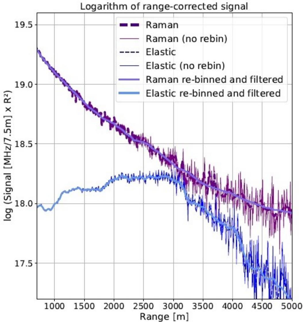
Figure 6: The corrected signal obtained in a clear day on 19th July 2018 with the Barcelona Raman-LIDAR launching 500 shots with the pulsed laser. Purple continuous line shows the Raman backscattered corrected signal with an applied Savitzky-Golay filter; the blue continuous line shows the elastic backscattered.
