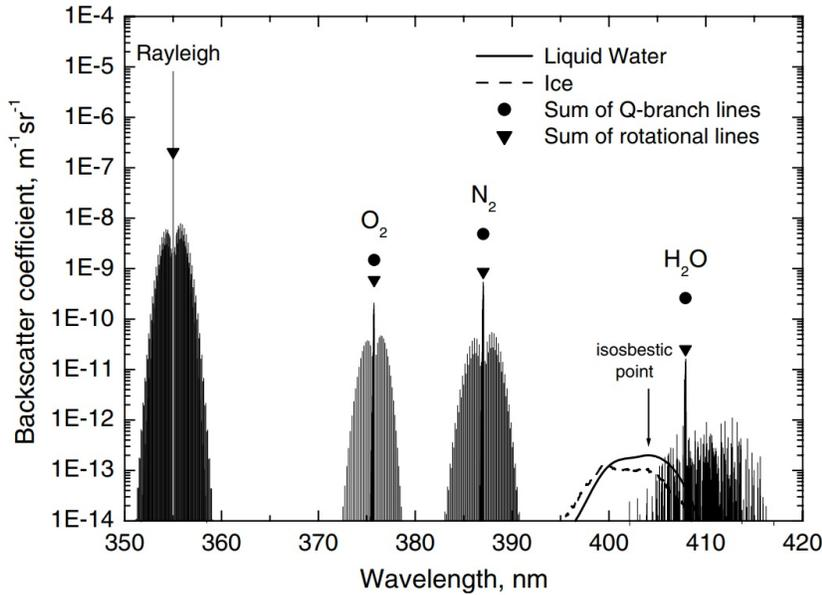
Figure 3: Figure that shows elastic and Raman backscattering coefficients as a wavelength function for basic atmosphere compounds. [10]
